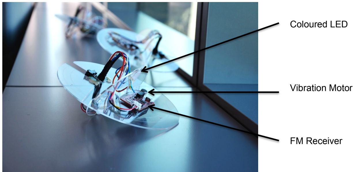
Figure 2: Internal, technical components of the Orb . Photo: Michael Smith
