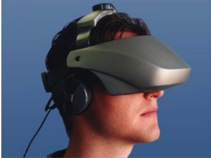
Figure 2: A Head Mounted Display (HMD) used for Virtual Reality (VR) to create immersive user environments. Image sourced: http://www.vrealities.com/products/head-mounted-displays/5dt-hmd-800
