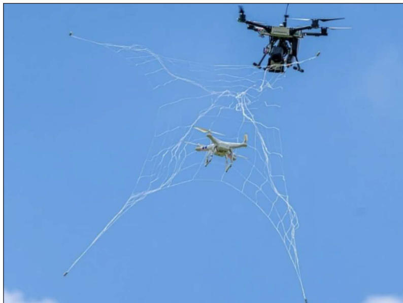
Figure 5: Ukrainian & Russian drones in a sky. DroneCatcher is a multicopter armed with a net gun. @airspaceview, 25 June 2024.
